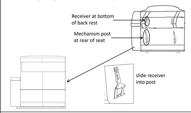
Step4: Connect the right hand facing recliner to the left hand facing recliner. Slide clips together then press the front and rear sides to ensure the clips are connected all the way to the bottom.
