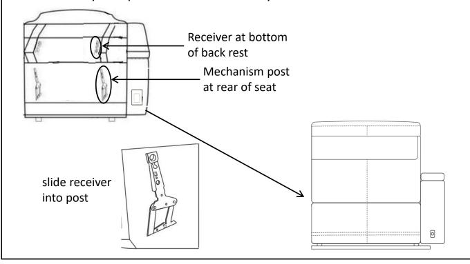
Step3: Keep back rest in an upright position then slide receivers into steel mechanism posts at seat of the right hand facing recliner, Press both sides of the back firmly into place to ensure it is fully locked.
