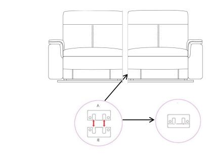
Step5: At the rear and base of lounge, connect the cords between the left hand facing recliner and the right hand facing recliner for electric reclining motion of the left and right recliners.
